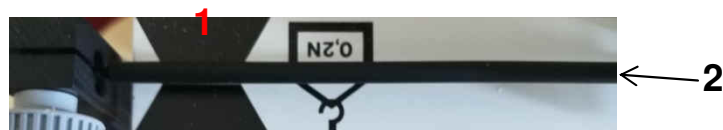
Fig. 2 Upper view on the frame aligned with the dynamometer at zero position (this is the magnified projection from the upper left hand corner of Fig. 1 (marked with X) . 1 – mark on the dynamometer, 2 – arm of the dynamometer
