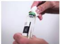
1. Take the bottle off from the incubator and mix carefully but not vigorously and then disinfect carefully the cap
